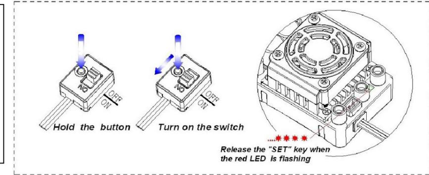
**Note2:** If you don't release the "SET" key as soon as the red LED begins to flash, the ESC will enter the program mode, in such a case, please switch off the ESC and re-calibrate the throttle range again from step A to step D.
